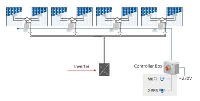
Note: The control box can convert AC 230V to DC 24V, and then control the working status of PEFS.
