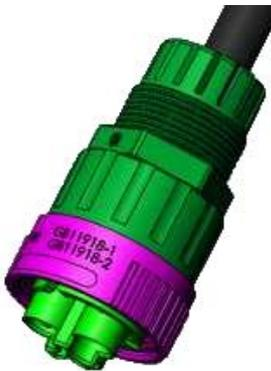
**Step 5:** Insert seal into body, then tighten the nut, torque  $1.5 \pm 0.3 \text{N}\cdot\text{m}$ . The maximum spacing between the nut and the body after tightening is 1.5mm.
