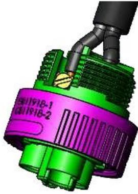
**Step 4:** Screw body to housing, tightening torque  $1.2 \pm 0.2 \text{N}\cdot\text{m}$ .
